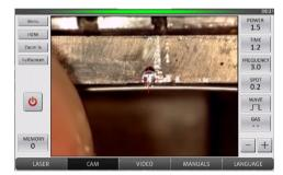
Every EASY is equipped with the so-called "EMBEDDED CAMERA SYSTEM". The images captured by the integrated HD-CAMERA, with no latency of sort, are displayed on the 10" LCD, where all the Working Parameters are always displayed. The ZOOM function allows digital magnification of 15x, 20x and 40x.
