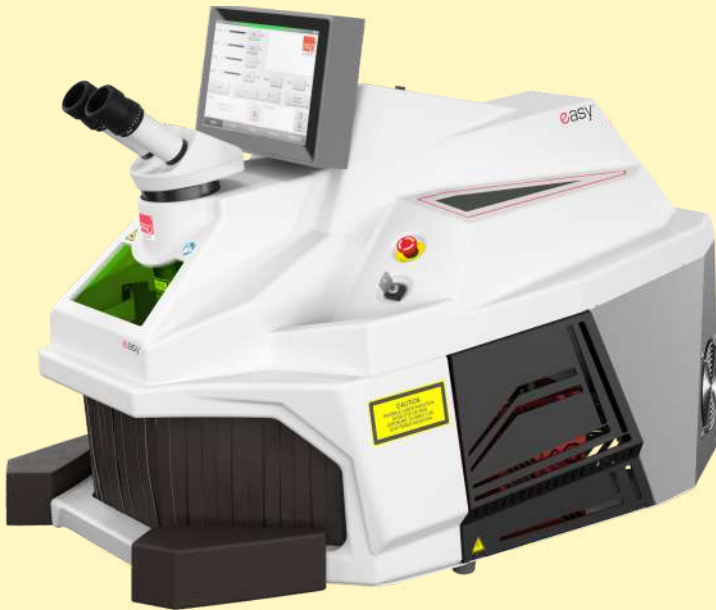
Sustained by a 6-LITERS LIQUID TANK, DUAL-RADIATOR Cooling System
